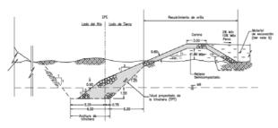
Figure 7: Trench fill revetment
