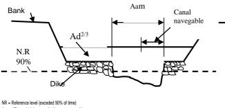
Aam = River width in controlled low water condition > navigation channel width.
