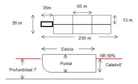
Figure 2: Design tow, plan view and profile
